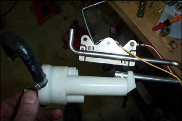
Figure 5 - Removing The Mixing Chamber
