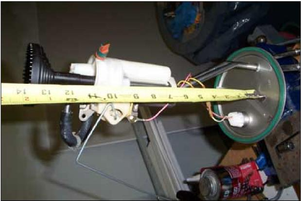
Figure 3 - Measuring The Factory Strainer Depth
