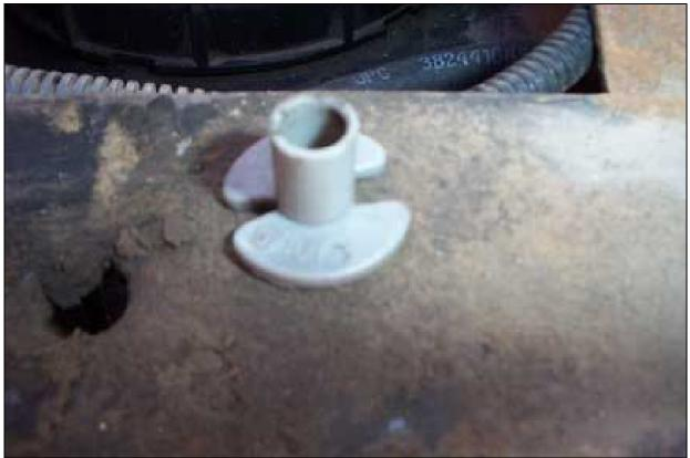
Figure 1- Line Release Tool
