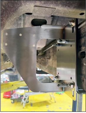
OUTSIDE / TIGHT TO FRAME / LOW POSITION INSIDE / BRACKET EXTENDED AWAY FROM FRAME **NOTE:** E-Brake cable should run through a split hose or sleeve, and not be pinched, if behind bracket.
